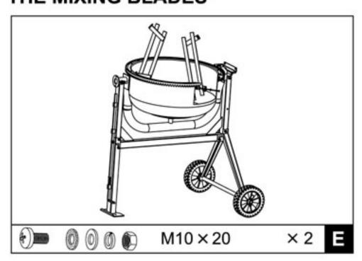
Mount the mixing blades inside the bottom drum loosely as shown - Two holes are provided at the base of the drum into which a M10X20 cross headed screw may be inserted from the outside. A leather washer, flat washer, lock washer and a nut should be threaded on loosely on the inside. The leather washer should be placed under the blade down against the drum.
